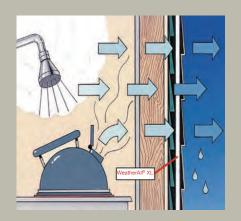
Perforated to enhance water vapor permeability. This important feature helps ensure that water vapor can escape the wall cavity. Trapped water vapor can cause mold formation and, if unnoticed, can lead to structural damage.
